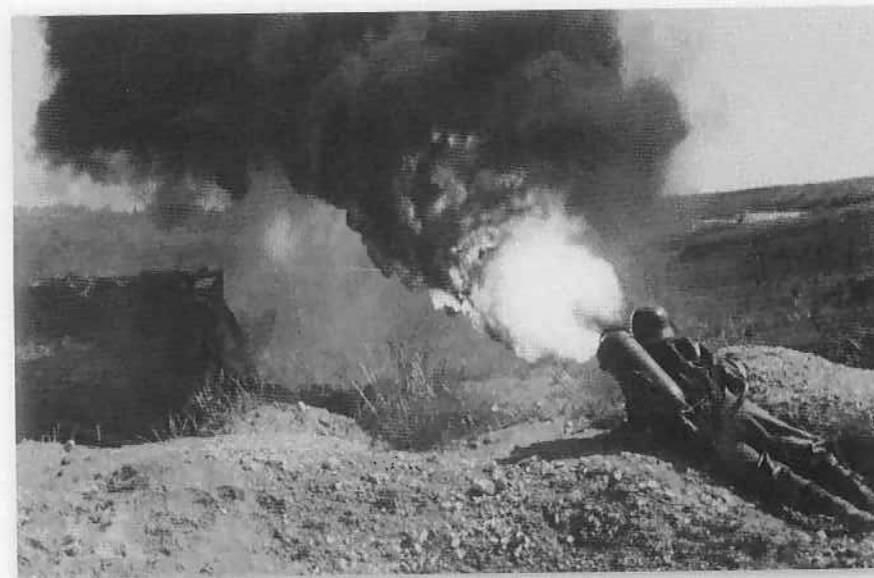
A German pioneer team attacking a Soviet position with a Flammenwerfer 41 flamethrower. Each pioneer battalion in LIV Corps had 10–12 flamethrowers, and they were particularly effective at driving Soviet troops out of underground bunkers. The Flammenwerfer 41 weighed 22kg and it had enough fuel for ten seconds of use; it had a maximum range of 30m. (HITM Photo Research)
